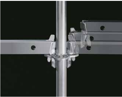
With the ledger assembly, the wedge falls into the opening of the rosette through its own force of gravity and locks automatically. The rosette node connection is extremely rigid with a high loading capacity.
