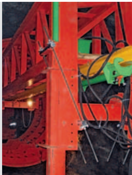
Optional VARIOKIT accessories such as hydraulic winches, electric drive units, lifting and lowering units and hydraulic cylinders for operating the wall and slab formwork elements are available in the VARIOKIT construction kit and, if necessary, are planned according to project requirements.
