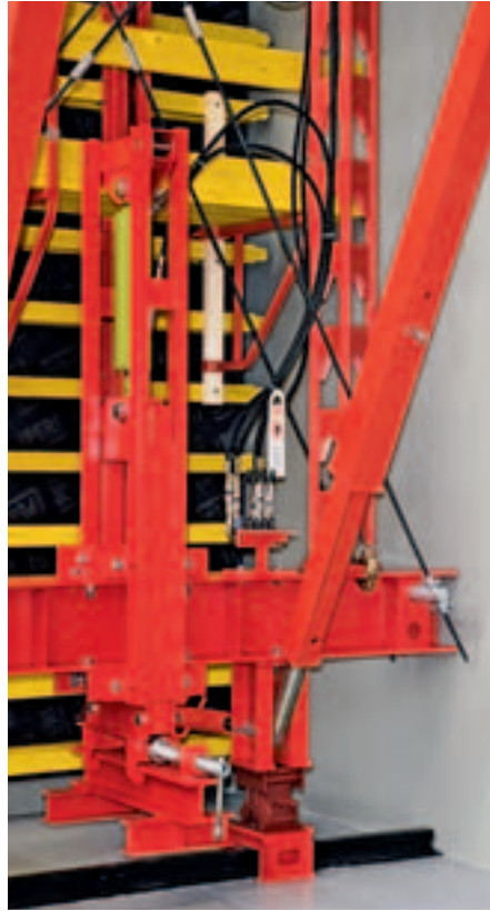
As an option, the tunnel formwork carriage can be equipped with the hydraulic lifting and lowering unit. In addition, the unit allows easy adjustment of the formwork to suit the particular gradient.
