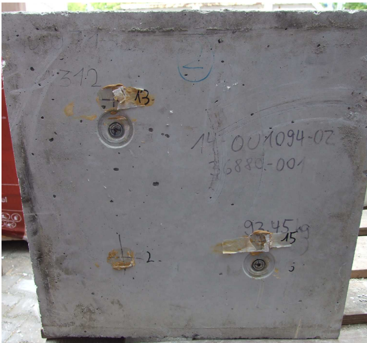
Photo 5 Unexposed face after fire test
