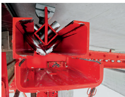
The track units roll self-centering over the roller units and rails along the bridge gradient.
