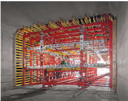
HD 200 Props as bracing: The heavy-duty props offset the horizontal loads generated from the concrete pressure; this avoids costly and time-consuming anchor solutions.
