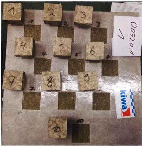
image 1: fracture pattern sample 1
