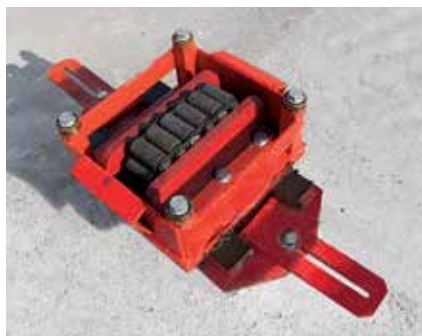
The carriage supporting shoe is mounted on the carriage supporting point and facilitates a smooth moving procedure.
