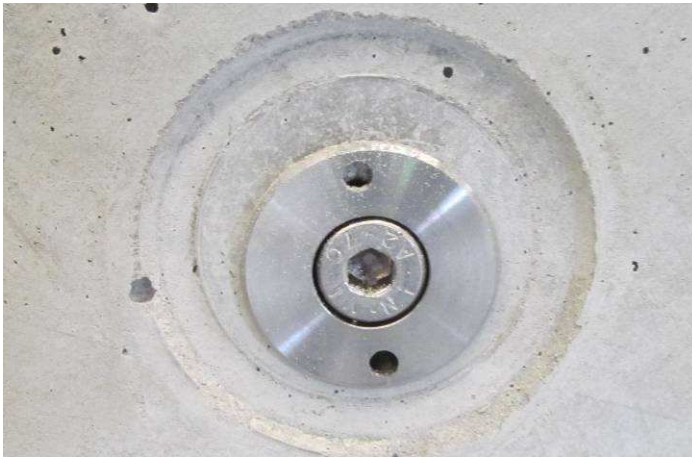
Photo 4 Screw plug "Schraubstopfen MX 15-50 MF-LS" Exposed face before fire test
