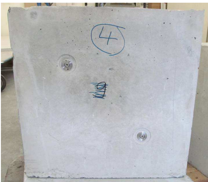
Photo 3 Exposed face before fire test
