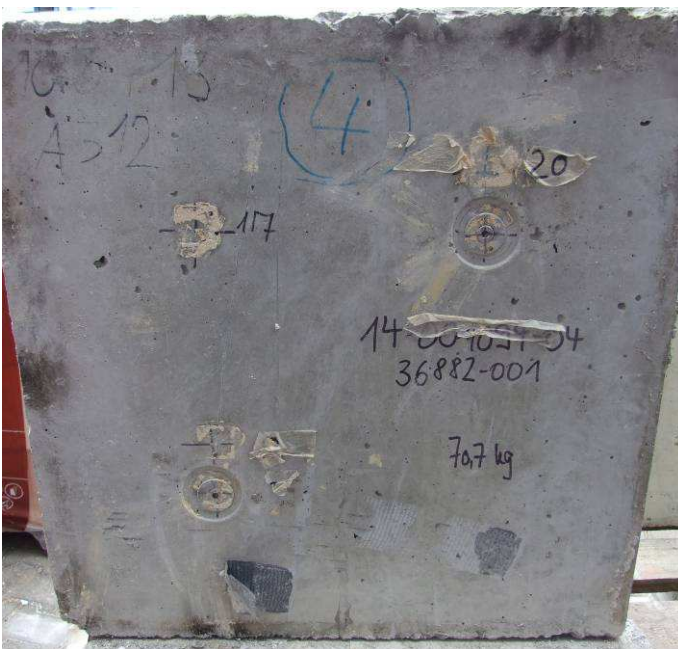
Photo 5 Unexposed face after fire test
