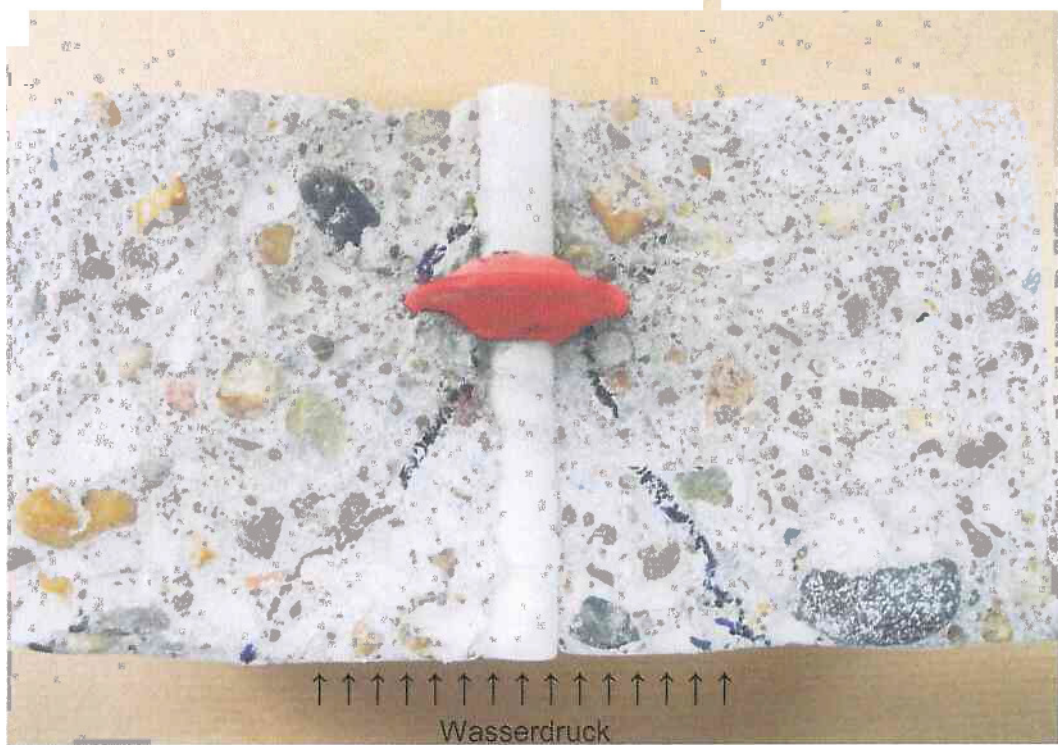
Picture A3: sample 2: glass fiber rod (ripped \varnothing = 14 mm)
