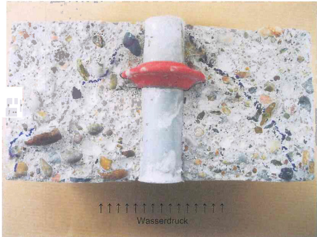
Picture A4: sample 3: plastic pipe (inner \varnothing = 22 mm, outer \varnothing = 26 mm)
